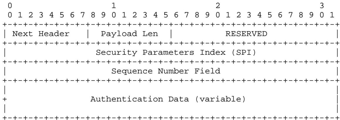
The following subsections define the fields that comprise the AH format. All the fields described here are mandatory, i.e., they are always present in the AH format and are included in the Integrity Check Value (ICV) computation (see Sections 2.6 and 3.3.3).
