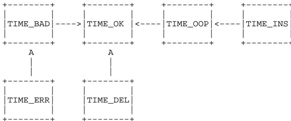
The state machine makes a transition once each second at an instant where the microseconds field of the kernel time variable overflows and one second is added to the seconds field. However, this condition is checked at each timer interrupt, which may not exactly coincide with the actual instant of overflow. This may lead to some interesting anomalies, such as a status indication of a leap second in progress (**TIME\_OOP**) when actually the leap second had already expired.
