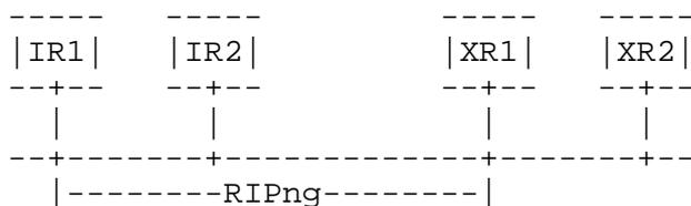
The Internal Routers (IR1 and IR2) are only running RIPng. The External Routers (XR1 and XR2) are both running BGP, for example; however, only XR1 is running BGP and RIPng. Since XR2 is not running RIPng, the IRs will not know of its existence and will never use it as a next hop, even if it is a better next hop than XR1. Of course, XR1 knows this and can indicate, via the Next Hop mechanism, that XR2 is the better next hop for some routes.
