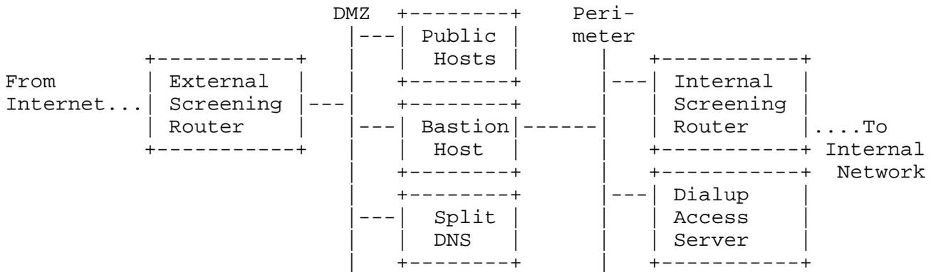
External screening routers typically have inbound access lists that block unauthorized traffic from the Internet, and outbound access lists that permit access only to DMZ servers and the bastion host. The inbound filters commonly block the Private Address Space, as well as address space from the enterprise's internal network. If the internal network address changes, the inbound filters clearly will need to change.
