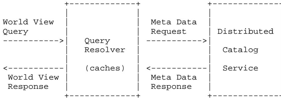
Figure 2: Components of a Nomenclator System
