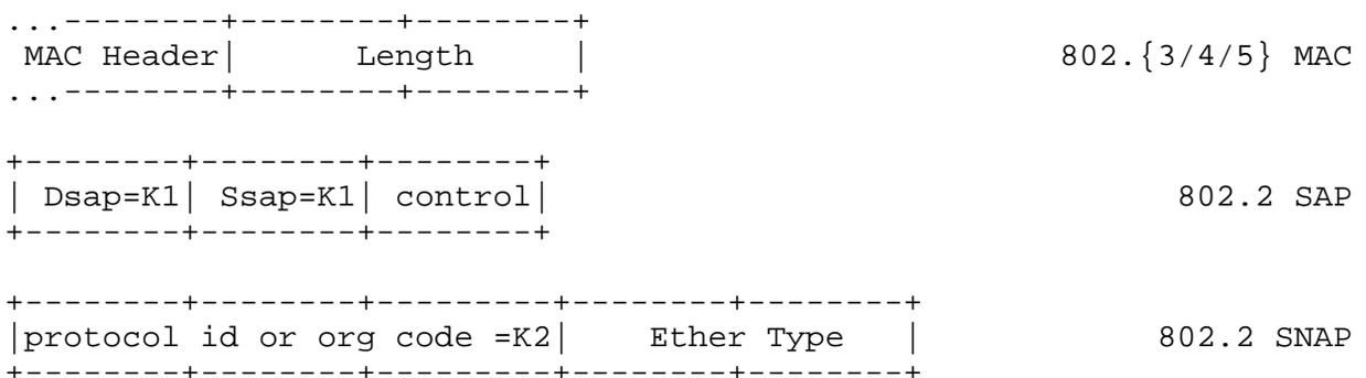
The total length of the SAP Header and the SNAP header is 8-octets, making the 802.2 protocol overhead come out on a nice boundary.
