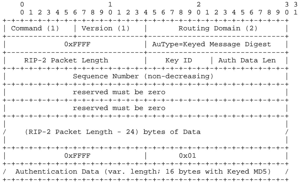
In memory, the following trailer is appended by the MD5 algorithm and treated as though it were part of the message.
