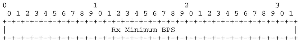
The Rx Minimum BPS is a 32 bit value indicating the speed in bits per second.
