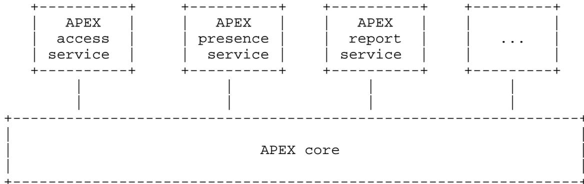
That is, applications communicate with an APEX service by exchanging data with a "well-known endpoint" (WKE).
