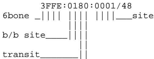
Note 1: the two sites numbered 0x001 in the above examples are really two different sites as their pNLA1 authority above them is different (i.e., in the first case no transit exists thus the site is directly connected to the pTLA backbone ISP, and in the second case the site is directly connected to intermediate transit ISP 0x80).
