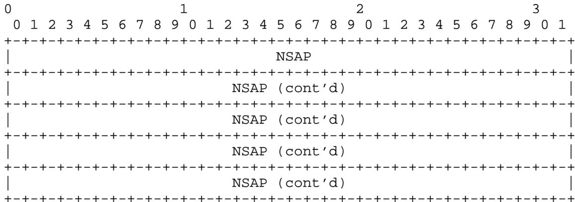
The Calling Number AVP MUST be encoded as a 20 octet binary encoded NSAP address when the B bit is set in the Bearer Type AVP. The NSAP binary encoded address provides a broader range of address encapsulation methods than an ASCII field. The structure of the NSAP address (e.g., E.164, ICD, DCC) is defined in [AESA].
