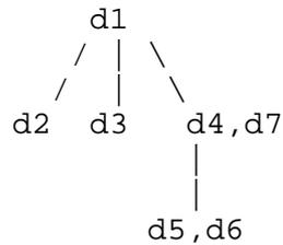
Next the algorithm visits the next segment, which is the one connecting d4, d5, and d6. Using the process stated above, d5 can eliminate d6, since it hears d4 on a different port from where it hears d6. Finally, the topology looks like:
