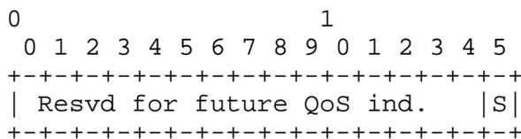
The Attribute Value field is a 16-bit mask, with one bit defined. The S bit indicates either non real time (S bit set to 0) or real time (S bit set to 1) service requirement. The other bit fields are reserved for future use.
