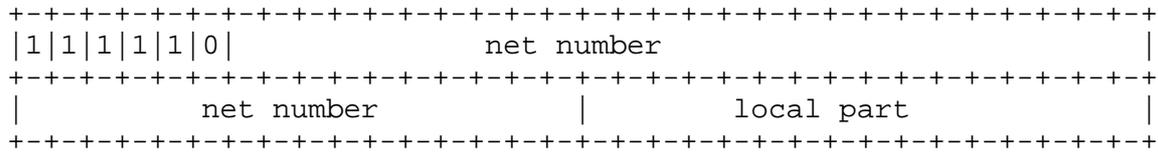
Class F-8G has the seven higher order bits set to 1111110, a 49 bit network number and a 8 bit host address.
