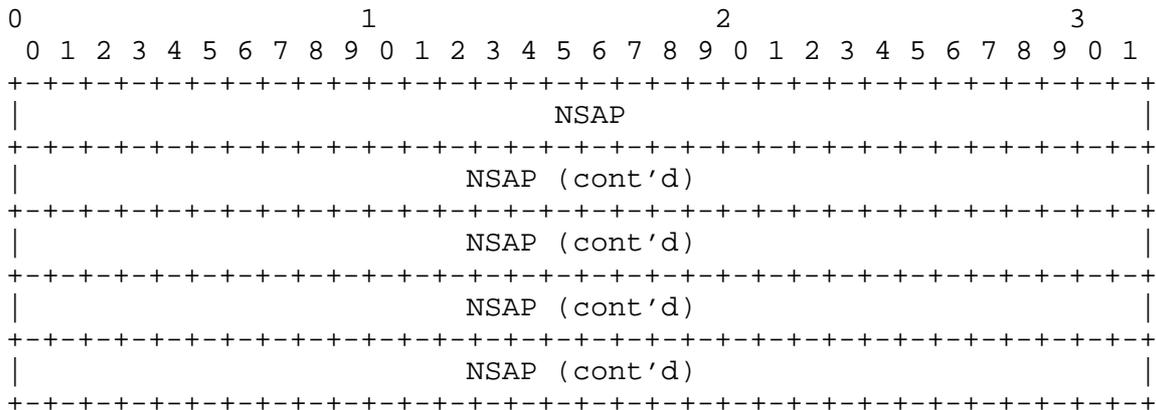
The Calling Sub-Address AVP MUST be encoded as a 20 octet binary encoded NSAP address when the B bit is set in the Bearer Type AVP. The NSAP binary encoded address provides a broader range of address encapsulation methods than an ASCII field. The structure of the NSAP address (e.g., E.164, ICD, DCC) is defined in [AESA].
