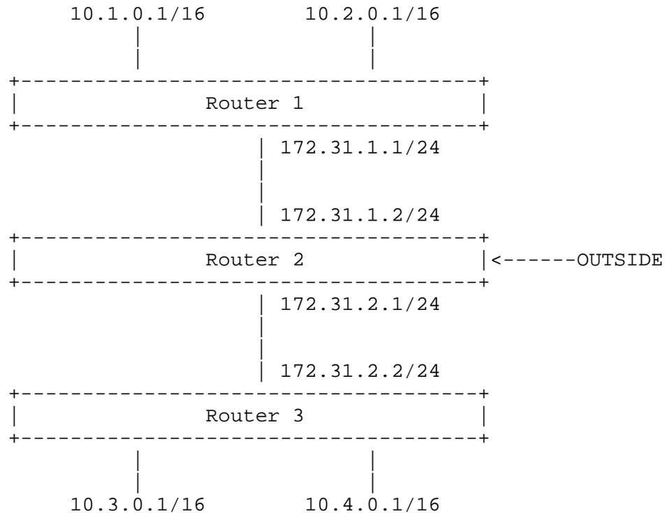
Router 1 can reach its two locally connected subnets, 10.1.0.0/16 and 10.2.0.0/16. It will aggregate them into a single announcement of 10.0.0.0/8 when it advertises out the 172.31.1.1 interface.
