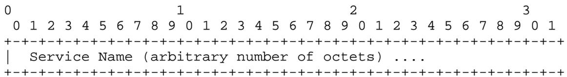
The Service Name is of arbitrary length, but must be at least 1 octet. The Service Name is UTF-8 encoded. [10646]
