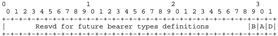
The bearer type AVP encodes the bearer type for the requested call. This document extends the bearer types with an indication of ATM bearer support (B-bit). If bit B is set, broadband access is requested (ATM). If bit A is set, analogue access is requested. If bit D is set, Digital access is requested.
