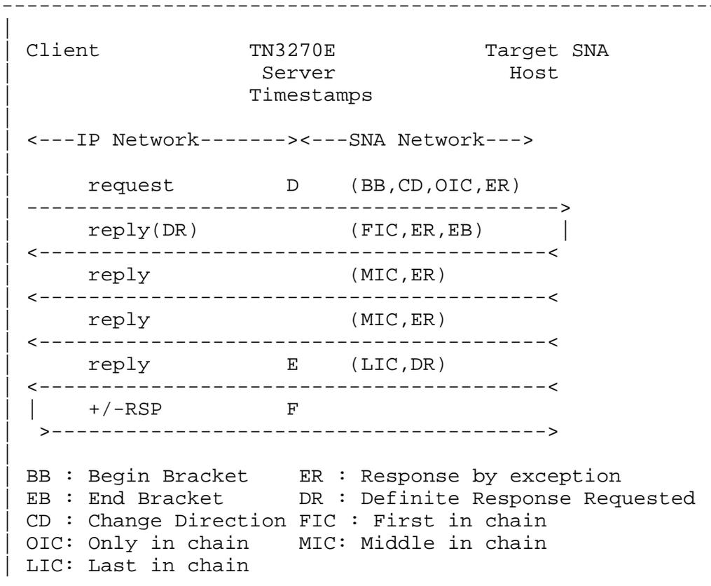
Timestamp D is taken at the TN3270E server when the server has received data from a client for forwarding to its target SNA host, and the direction of the SNA session allows the server to forward the data immediately (either the direction is inbound towards the SNA host, or the session is between brackets). This is most likely when the server finds the end of record indicator in the TCP data received from the client.
