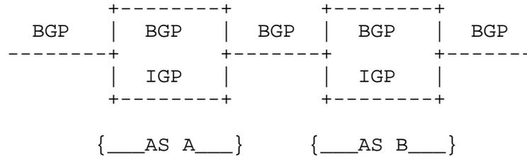
This diagram points out that, while BGP alone carries information between ASs, a combination of BGP and an IGP carries information across an AS. Ensuring consistency of routing information between BGP and an IGP within an AS is a significant issue and is discussed at length later in this paper.
