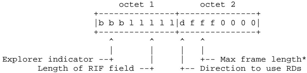
\* Note that the length of the Maximum frame length subfield has recently been extended to 6 bits.
