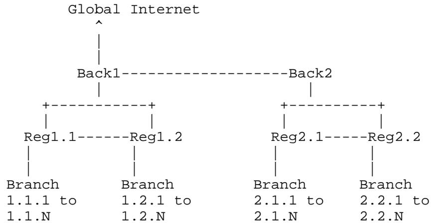
In this drawing, assume Back1 and Back2 exchange full routes; Back1 is also the exterior router. Regional routers (Reg) exchange full routes with one another and aggregate addresses to the backbone routers. Branch routers default to regional routers.
