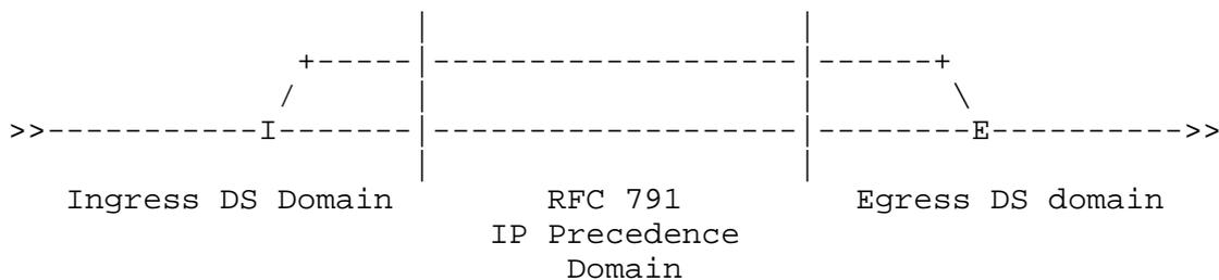
In this situation, the DS edge node for the egress domain (i.e., the node at the right-hand vertical line) can select the appropriate AF group (e.g., via an MF classifier), but cannot reconstruct the drop precedence information that was removed from the outer header when it
