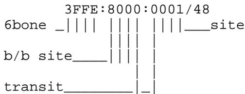
Another example of this usage, assuming the same backbone pTLA1 of 0x800 and an intermediate transit ISP under it (numbering from the left edge) with an NLA1 of 0x80, and a sequential site ID of 0x0001, the routing prefix for the first site connected would look like:
