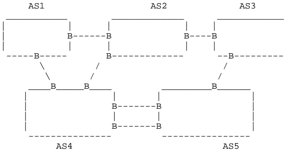
Here, ASs exchange standardized routing information via border nodes B. Under this model, each AS can itself consist of a set of interconnected ASs, with standardized routing interaction. Thus, the interdomain routing model is hierarchical. Also, each lowest level AS employs an intradomain QoS-based routing scheme (proprietary or standardized by intradomain routing efforts such as QOSPF). Given this structure, some questions that arise are:
