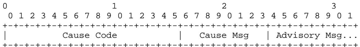
The Cause code is not changed from [RFC2661], except for the fact that it can also carry Cause Codes specific to ATM signalling messages, these cause codes can be found in ATM
