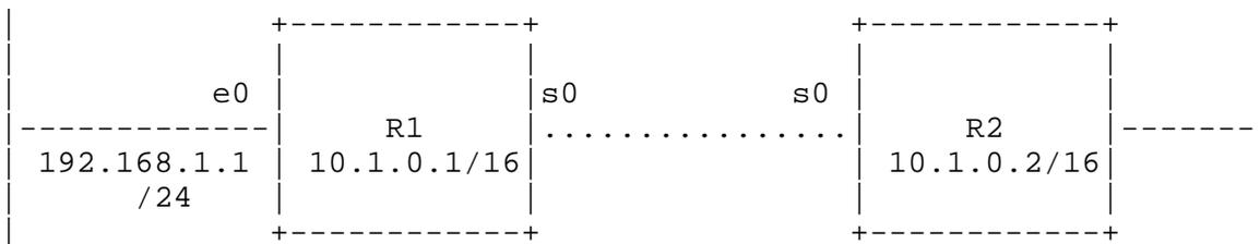
In the above example, software in routers R1 and R2 automatically forward every packet received on serial interface S0 to Ethernet interface E0. They forward every packet on e0 to their local S0. Neither S0 has an IP address. R1 has the router ID 10.1.0.1/16 and R2 has 10.1.0.2/16.
