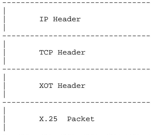
RFC convention is that a packet format is represented graphically with the data sent first above the data sent later. This convention is followed in this document, and therefore, while we refer to X.25 being transported over TCP, we draw the packet format with the X.25 portion of the packet lower on the page than the TCP portion.
