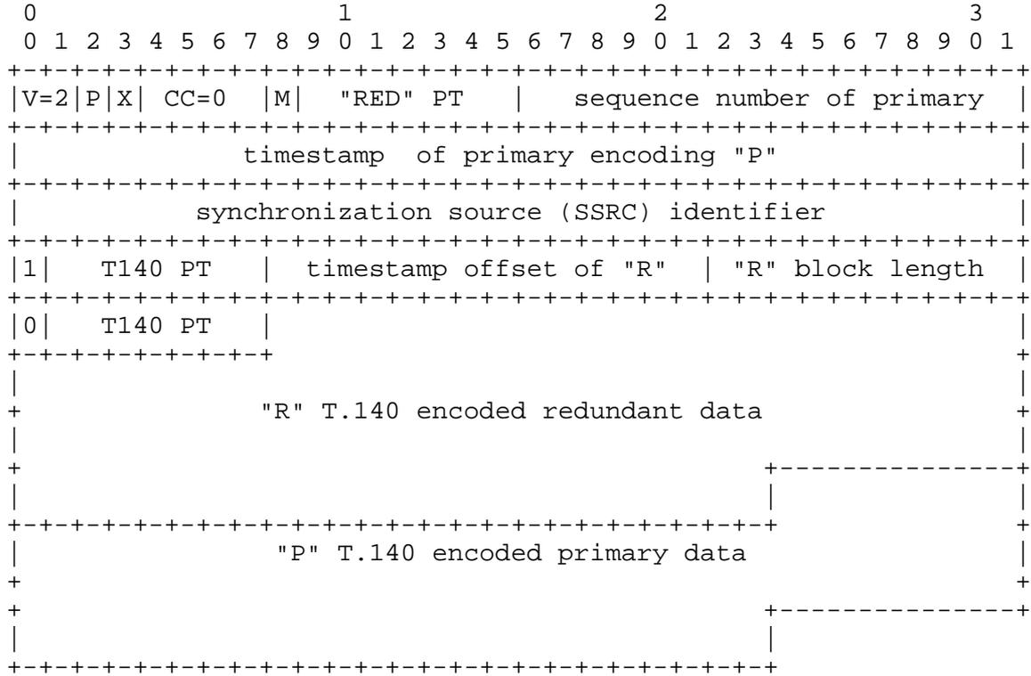
Figure: Examples of RTP text packets.
