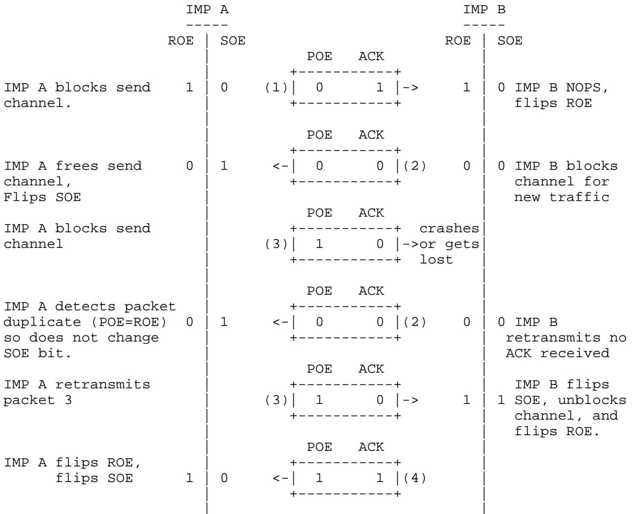
In fact each send/receive module has 8 OE bits, so up to 8 packets can be outstanding in either direction.
