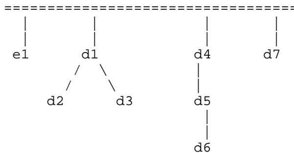
In the above case, we would give d1, d4, and d7 a chance to show that e1 is not really on that segment. d4 and d7 hear e1 on the same port which connects them to that segment, so they cannot eliminate e1 from the segment. However, d1 will hear e1 on a different port, so we move e1 down onto the segment which is connected by that port. This yields the following:
