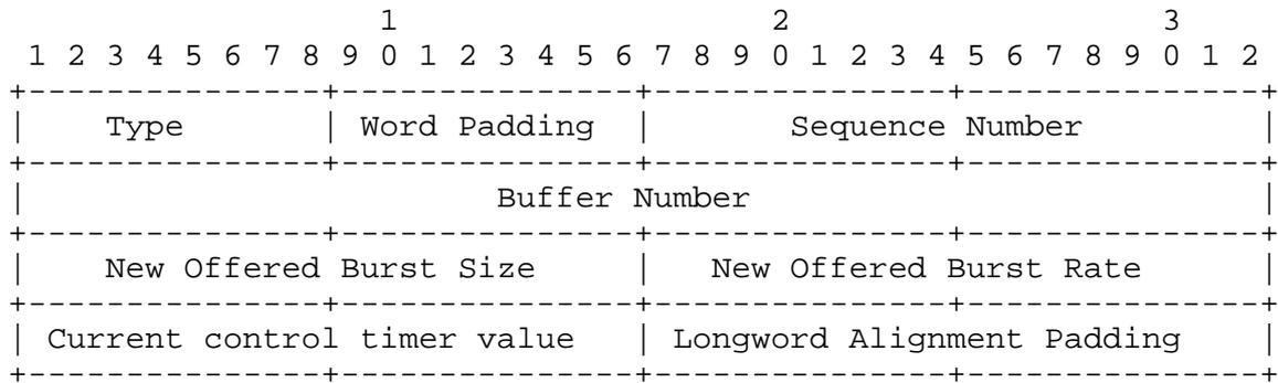
New offered burst size: burst size for subsequent buffer transfers, possibly based on performance information for previous buffer transfers.
