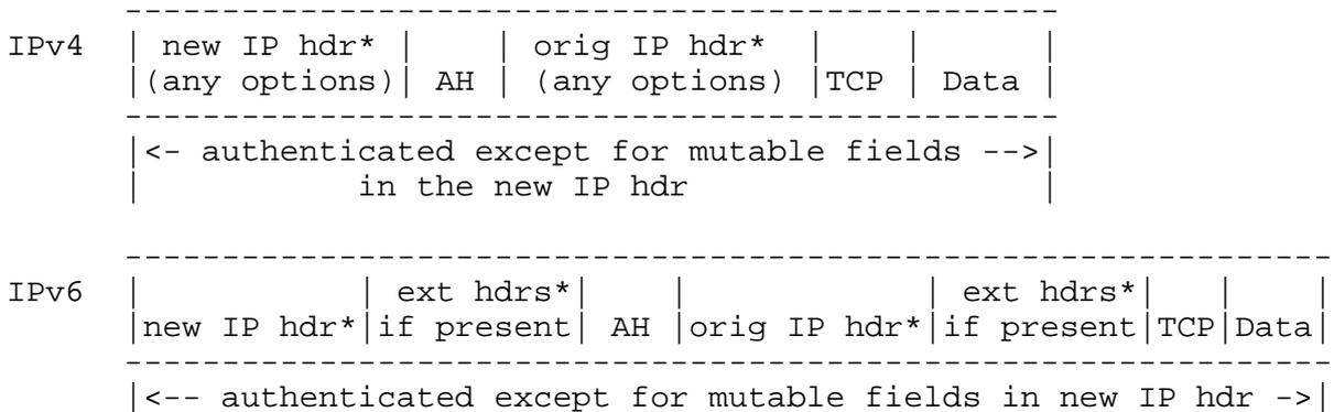
\* = construction of outer IP hdr/extensions and modification of inner IP hdr/extensions is discussed below.
