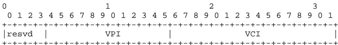
The VPI/VCI identifier is a 32 bit value encoding the VPI(12 bits) and VCI (16 bits) value.
