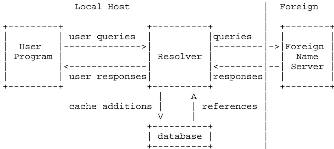
User programs interact with the domain name space through resolvers; the format of user queries and user responses is specific to the host and its operating system. User queries will typically be operating system calls, and the resolver and its database will be part of the host operating system. Less capable hosts may choose to implement the resolver as a subroutine to be linked in with every program that needs its services.
