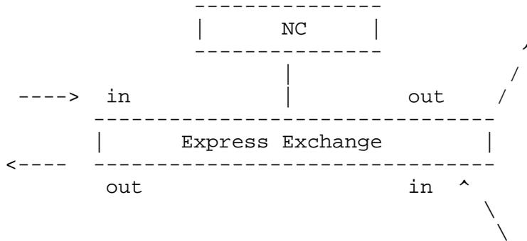
The above figure illustrates the two major functions with messages travelling in both directions and directly through the Express Exchange, except in the case of messages that must be acted on by the Net Controller. These messages will be explained in detail later.
