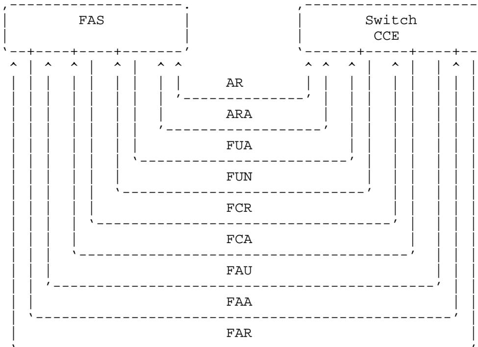
When a connection is established, periodically during the course of maintaining the connection and when a change in connection state occurs, the switch CCE sends a Flow Update Notification (FUN) message to the FAS. The FAS, in turn, responds with a Flow Update Acknowledge (FUA) message with a Flow failure code if an error condition has been detected. An example of error conditions would be receipt of a FUN message indicating octets received and sent for a connection never admitted.
